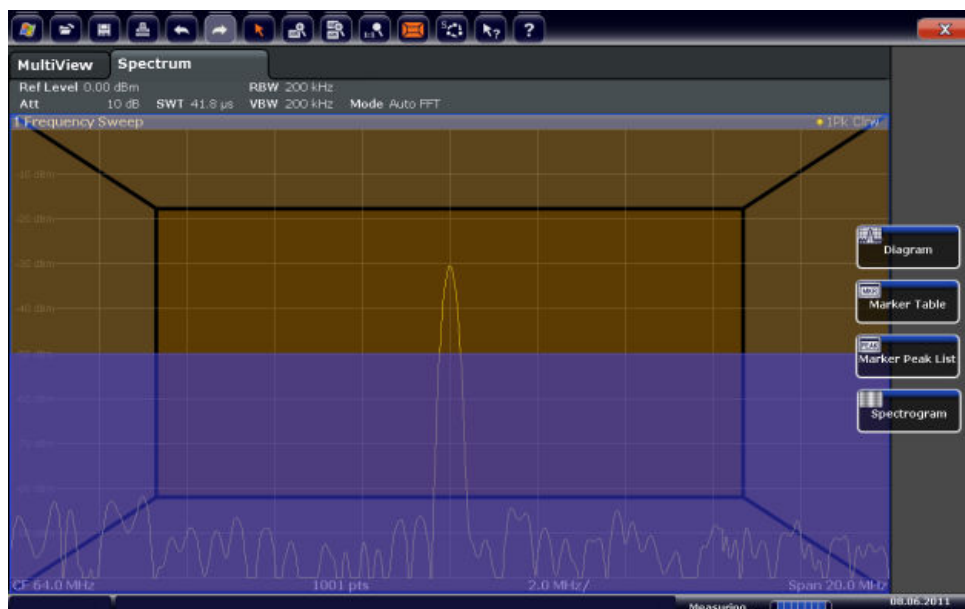
Figure 4-3: Adding a Spectrogram to the display
