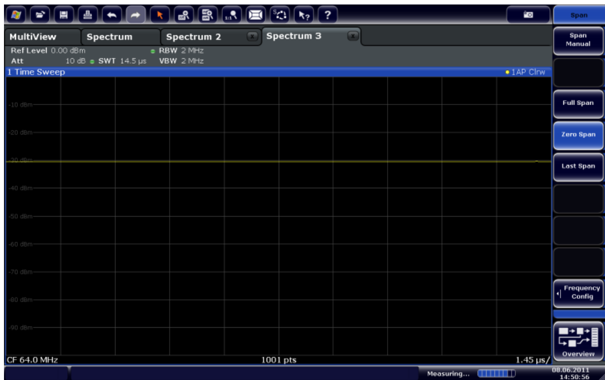
Figure 4-7: Time domain display of the calibration signal
