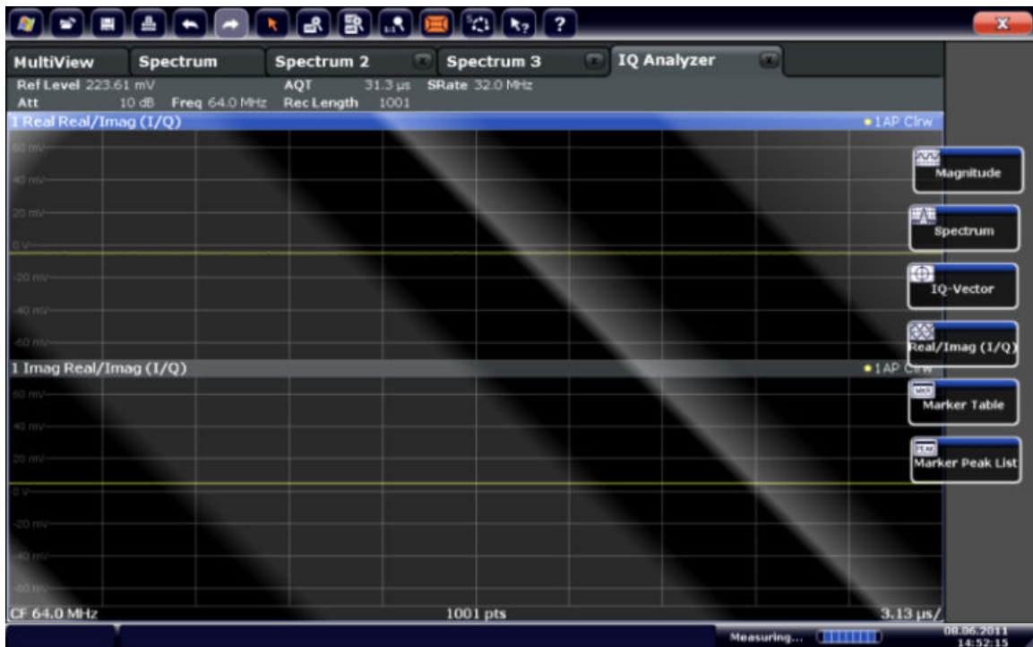
Figure 4-8: Inserting a Real/Imag diagram for I/Q analysis
